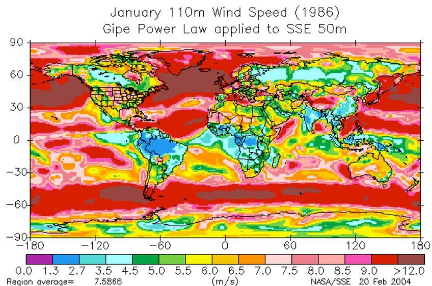
Figure 2: Gipe power law applied to the SSE 50-meter wind speed to elevate it to 110 meters over grassland surface representative of airports.
