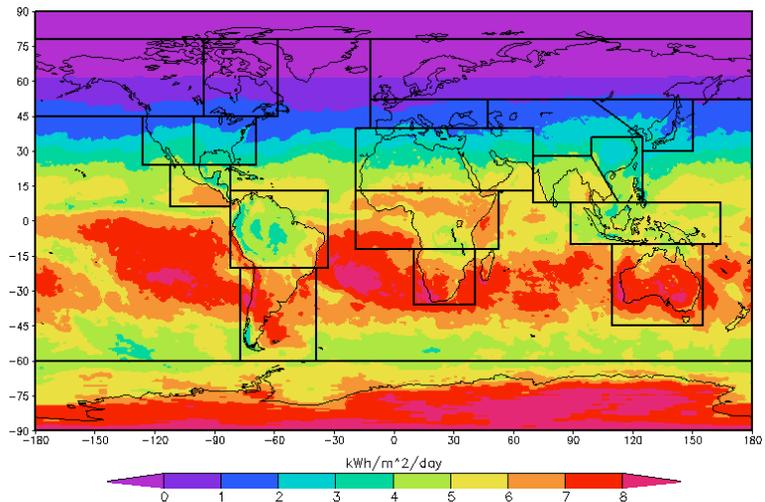
*Figure 1: Surface solar insolation for January 1986 from the latest run of the GEWEX SRB SW algorithm converted to SSE format. Outlined in black are land surface regions within which surface measurements are compared to the satellite based estimates for validation and assessment.*
