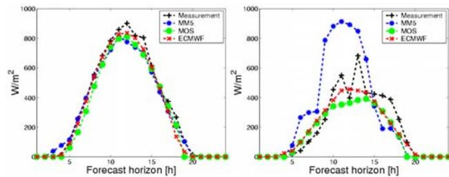
Figure 3: Comparison of different forecast approaches to ground measured irradiance for two test days (June 9 and 16, Germany). (3)
